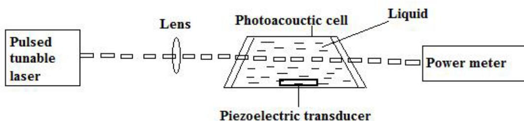
**Fig 9. Photoacoustic detection in liquids**
