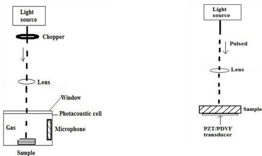
**Fig.8: Typical experimental arrangements used for photoacoustic studies on solids.**
