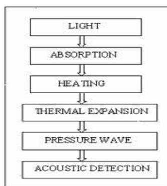
**Fig. 2: Principle of photoacoustics experiment**
