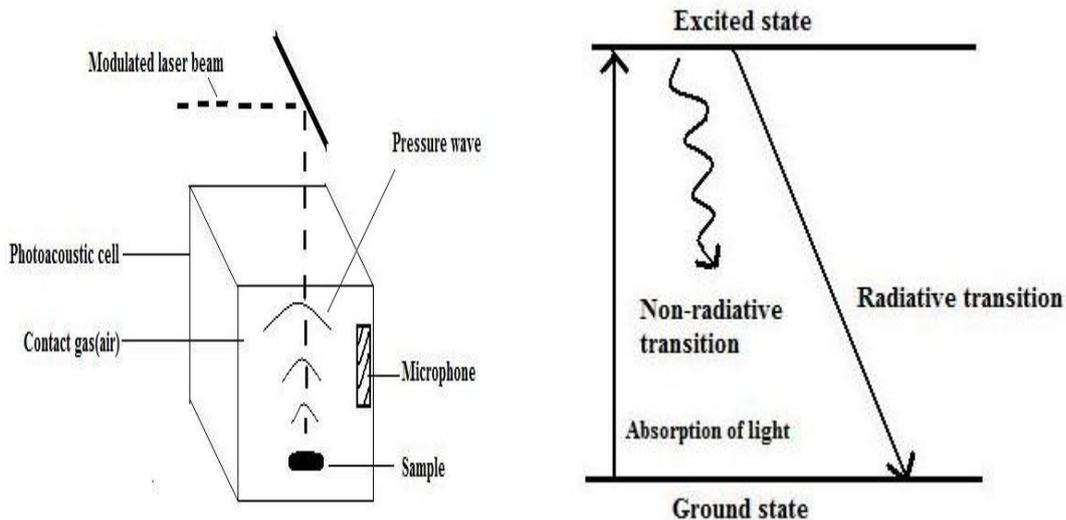
**Fig 7. Photoacoustic effect from a sample**
