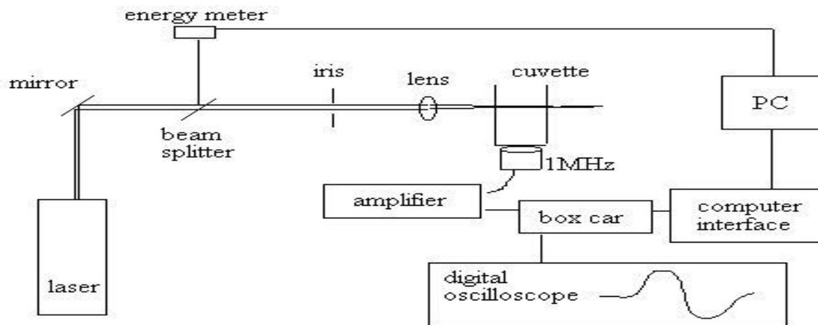
**Fig. 6: Instrumentation**
