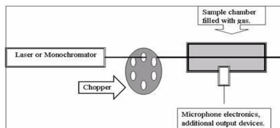
**Fig 4. Photoacoustic spectroscopy on a gas**
