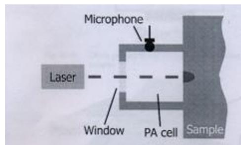
**Fig. 3 Indirect generation of photoacoustic waves for the analysis of solid and liquid samples**
